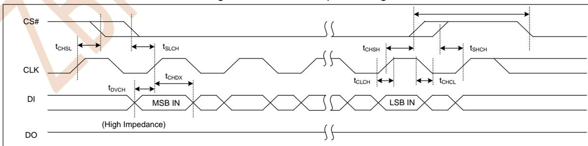
Figure 8.5 Input Timing
