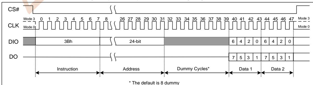
Figure 7.11 Fast Read Dual Output Instruction Sequence Diagram
