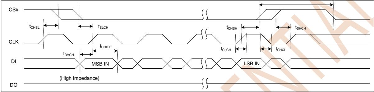
Figure 8.5 Input Timing
