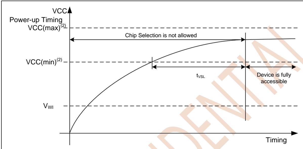
Figure 8.1 Power-up Timing
